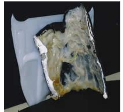
Fig. 2—Processors must beware of prolonged idle periods that can lead to oxidation and extreme burning of HDPE left in a hot machine barrel or head.
