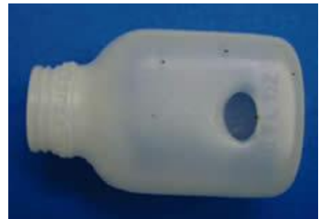
Fig. 1—As shown here, oxidized resin can cause not only black specks but blow-outs in
