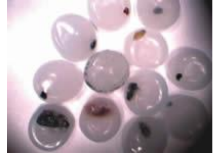
Fig. 3—Make sure that no oxidation has occurred before the pellets even get into the blow molding machine. Check your incoming resin for evidence of oxidation during pelletizing.
