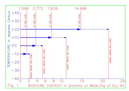
One kg [2.2lb] of dry air at sea level and  $10^{\circ}$ C [50°F] can be saturated with 7.626g [117.68 Grains] of moisture.
