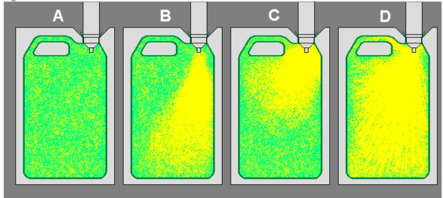
The air exchange is started after the initial blow of the preform with stagnant air. The initial blow time is set to be just long enough to stretch the preform to the shape of the cavity and vent all the ambient air between the product and the mold cavity. The product is finally vented before the mold is opened.
