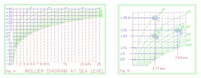
Point {A} in Fig. 5 represents air at a sea level with a temperature of 20°C [68°F], a moisture content of 3.77g/kg [58.17Grains] and a relative humidity of 25.7%. Cooling this air down to a temperature of 0°C [32°F] will raise its relative humidity to a value of 100% and the air would be saturated at this temperature. The air at point {A} has a dew point of 0°C [32°F].
