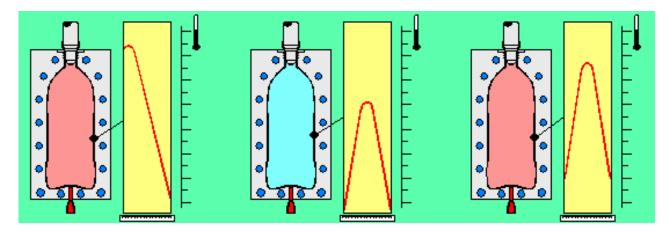
A specific point was chosen to measure the difference and the temperature profile was measured across the wall of the product at this point. A dramatic difference in the temperature between the inner and the outer surfaces was detected.
