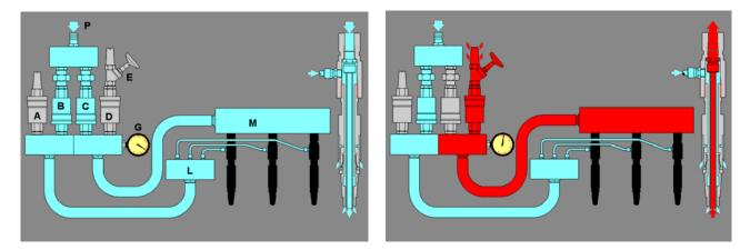
The illustration to the left below shows the valves  $\{B\}$  and  $\{D\}$  are opened while  $\{A\}$  and  $\{C\}$  are closed. The air now flows to the outer channel of the blow pin through the distributor  $\{L\}$ , washes the bottle removing heat from the inner surfaces and flows back through the inner channel of the blow pin through the machines manifold  $\{M\}$  to the throttle valve  $\{E\}$  and then finally vented out. The gauge shows
