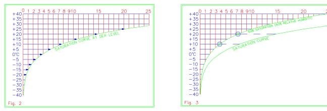
The relative humidity of the air represents the amount of moisture contained in the air related to the amount of moisture, which would saturate the air at the given temperature and pressure.
