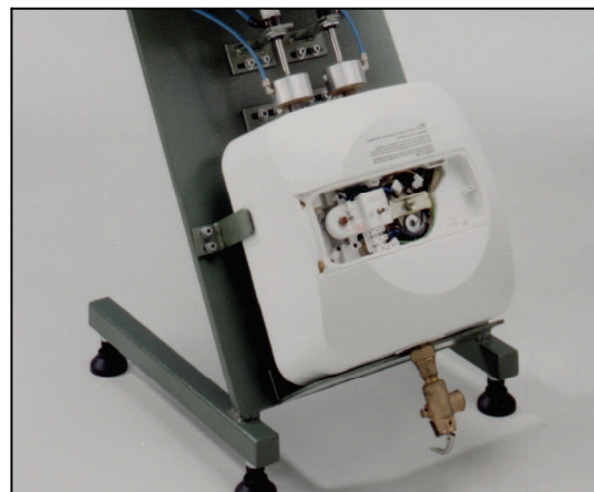
Leak testing a water heater
